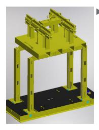
Direct loading crossbeams eliminate the use of complex nut housings. The load is directly transferred to the top of the lifting nut minimizing side loading on the jacking assemblies.
